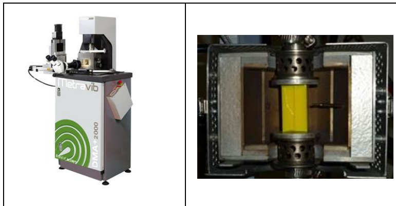
Metravib DMA and close up on a test fixture in thermal chamber
